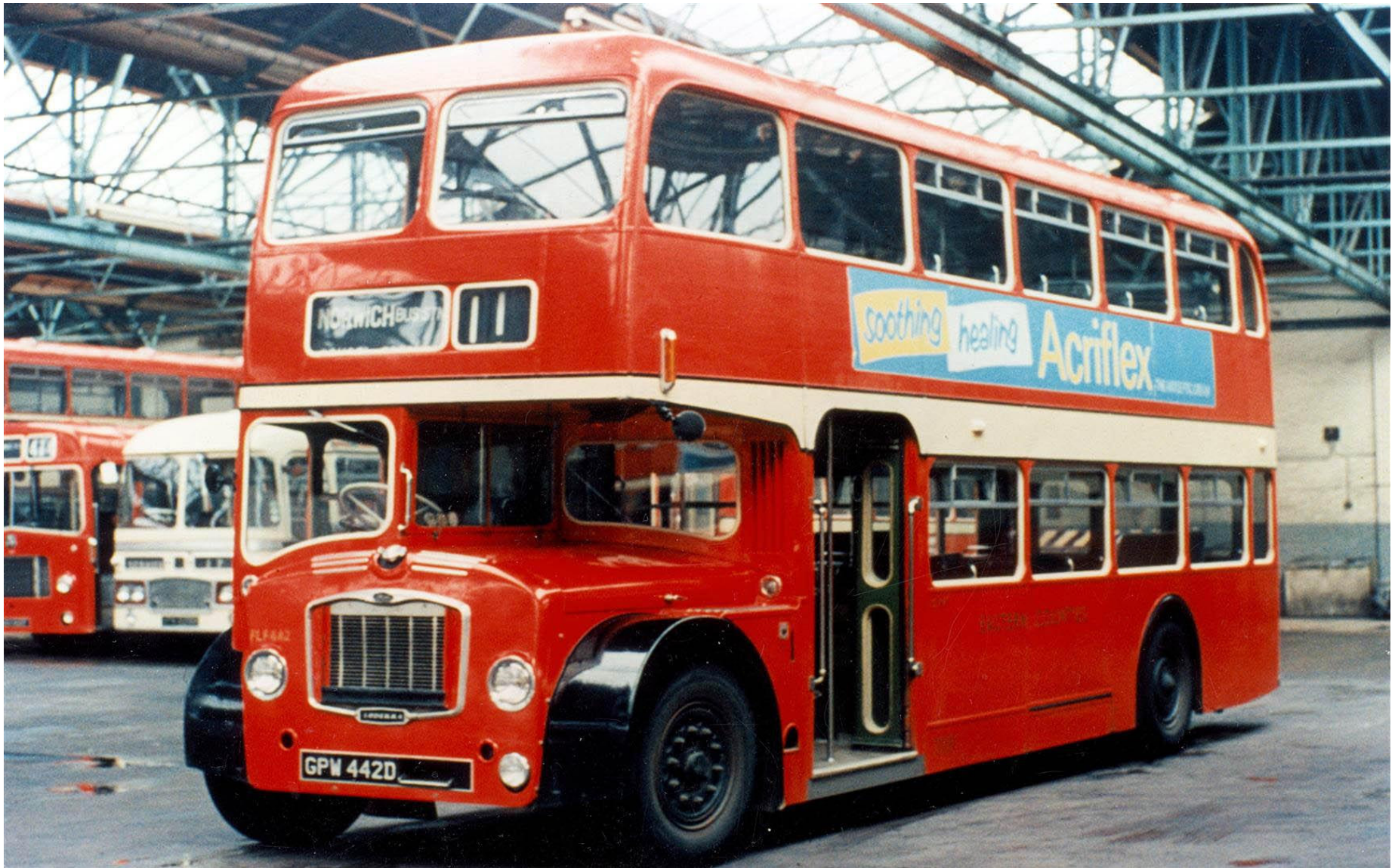
FLF 442 (GPW 442D) was a Bristol FLF6G Lodekka with an Eastern Coach Works 70 seat forward entrance body and was one of a class of 83 such vehicles delivered new to the company between 1966 and 1968. All the E, F and G suffixed members of this class with their upgraded 6LX engines were swapped for VRT models from the Scottish Bus Group during 1973, which many feel was a very bad move on the part of the National Bus Company, which by this time, had overall control of Eastern Counties operations. The bus is seen here when nearly new looking resplendent in 'Tilling' red and cream in the Surrey Street garage. Withdrawal came in 1982.
