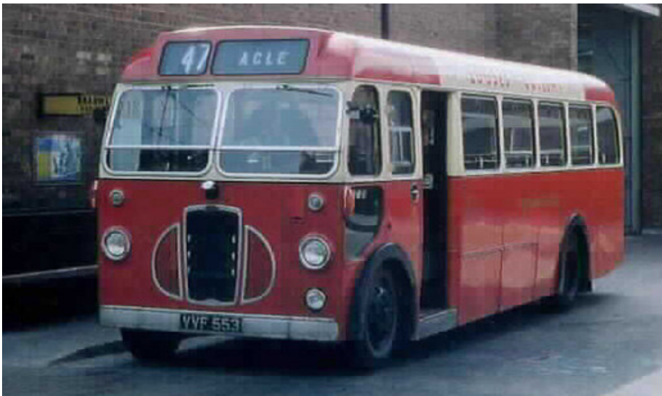
LC 553 (VVF 553) awaiting departure to Acle via Runham and Stokesby at Great Yarmouth Wellington Road Bus Station around 1969/70. This typical example of a Bristol SC4LK 35 seater saloon dates from 1957. Eastern Counties acquired a large fleet of these light weight saloons mainly for use on rural routes. LC 553 was the last of the 1957 batch and was withdrawn in 1970 after 13 years service.
