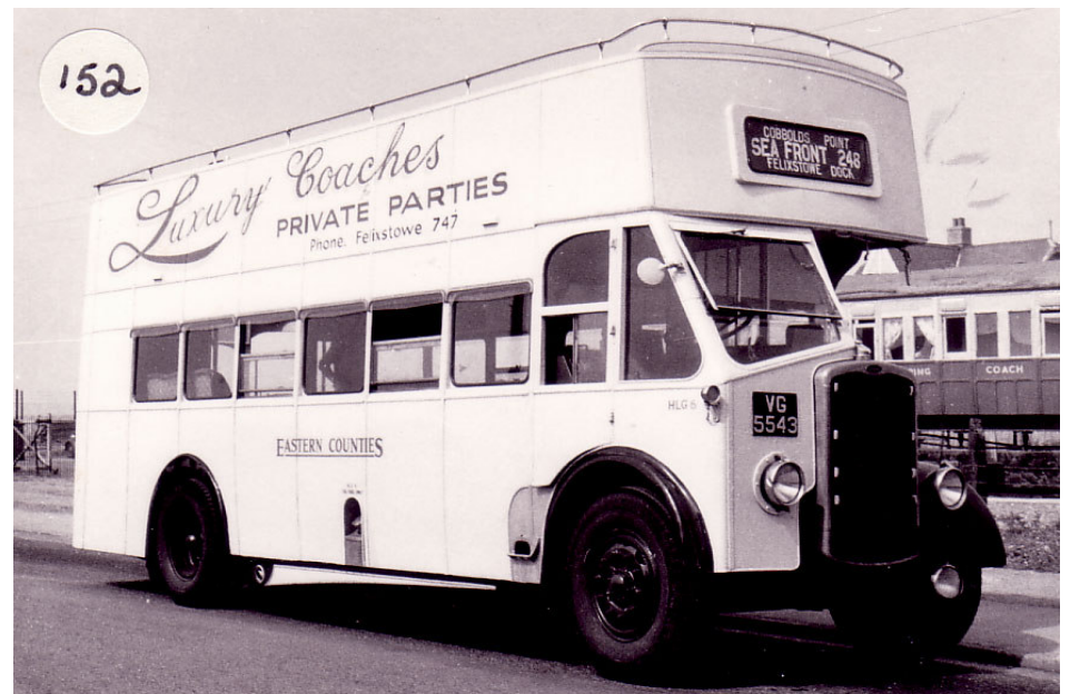
LG 6 (VG 5543) was one of a batch of eight Bristol GJWs delivered to Norwich Omnibus Company in 1933. LG6 passed to ECOC in 1935 and was converted to open top in 1950 to operate sea front services in Felixstowe. She remained in this guise for ten years until withdrawal in 1960. Photo: courtesy of Robert Mack.
