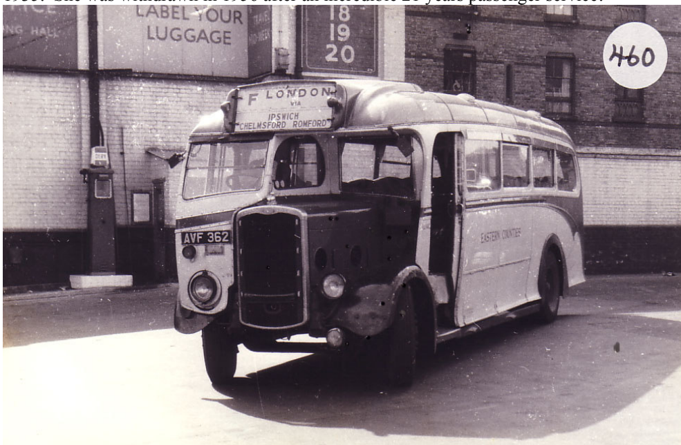
LJ 12 (AVF 362) was a 30 seat forward entrance ECW bodied Bristol JO5G coach. This splendid example was caught by the camera in London Victoria coach station having arrived from Lowestoft on express service F. She was one of ten JO5G coaches delivered during 1936 for express and private hire use. LJ 12 (later LJ 442) was withdrawn in 1956 after 20 years loyal service. Photo: courtesy of M. Mogridge.
