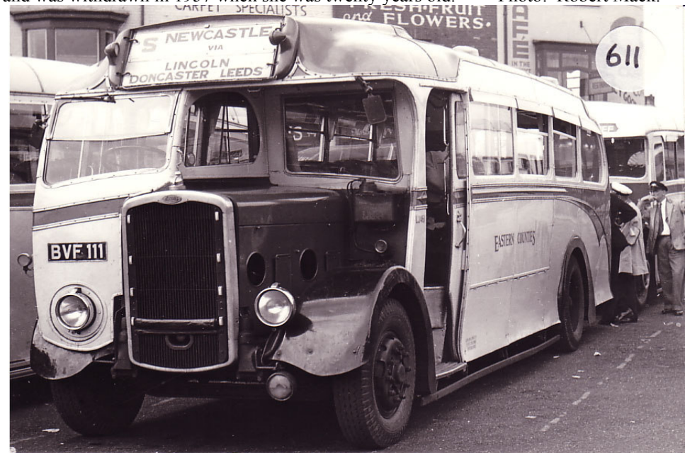
LJ 31 (BVF 111) was another of the 1937 delivery of 18 Bristol JO5G and JO6A 28 and 30 seat forward entrance ECW bodied coaches. LJ 31 (later LJ 461) is a JO5G and is seen here at rest in Doncaster in the early 1950s, breaking her journey on the long distance express service S from Lowestoft to Newcastle. She was withdrawn in 1954 after 17 years revenue earning service. Photo: courtesy of Robert Mack.
