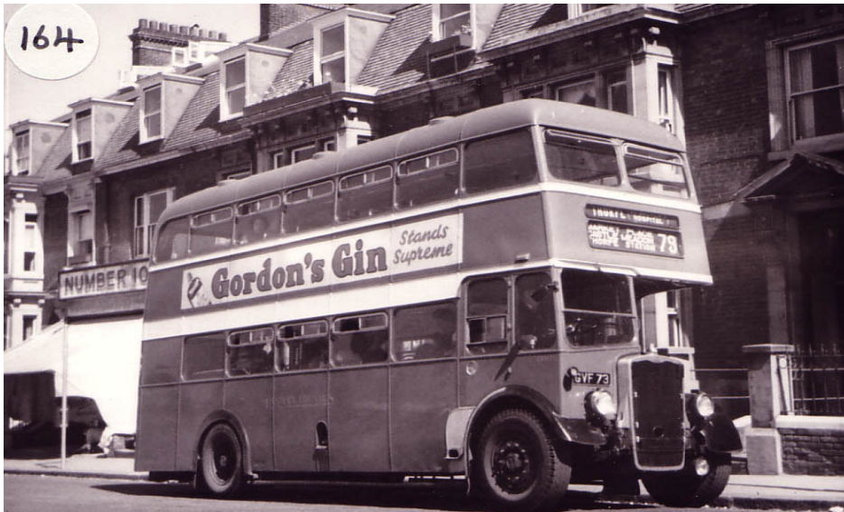
LKH 73 (GVF 73) was one of a batch of three 56 seat Bristol K6Bs with ECW bodies delivered to Eastern Counties in 1948. LKH 73 was later renumbered LKH 398 in 1963. She was caught by the camera near Norwich Thorpe railway station on a sunny day in the mid 1950s whilst operating on local service 79 to Thorpe St Andrew. She was withdrawn in 1967 after 19 years loyal passenger service.
