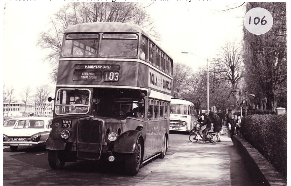
LKH 310 (MAH 310) was one of a batch of nine eight foot wide ECW bodied Bristol KSW5Gs with a seating capacity of 60. They were delivered new to the company in 1952. This mid 1960s shot captures LKH 310 in Cambridge, operating route 103 to Pampisford via Shelford & Stapleford. She was withdrawn in 1970 just prior to the NBC days.
