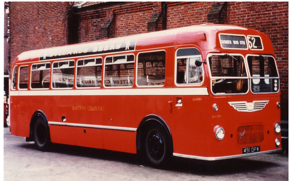
LM 491 (491 DPW) was one of a batch of four MW5G stage carriage saloons delivered to ECOC in 1963. These were Mk3 MWs seating 45 passengers and with fluorescent internal lights and hopper style ventilators. LM 491 was withdrawn in 1977 after 14 years service. She is seen here in Cromer's Cadogan Road bus station in the early 1960s, resplendent in Tilling red and cream livery. Photo courtesy of Malcolm King.
