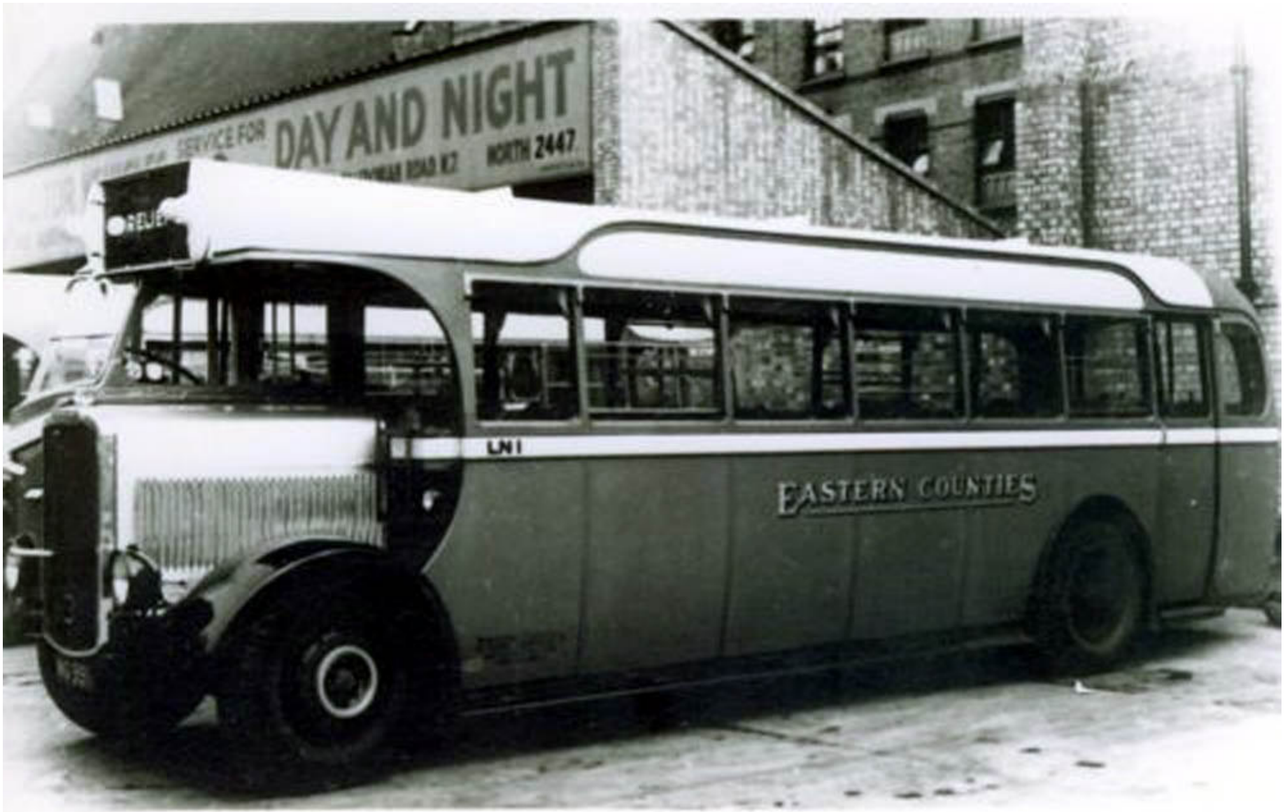
LN 1 (NG 9911) is a Bristol JNW with a 36 seat Eastern Counties Omnibus Company rear entrance body. This was one of a batch of ten such vehicles delivered new to the company in 1935. These vehicles were powered by the preferred Gardner oil engines which were very economical in operation, a point much favoured by the company management. All members of the class were re-numbered in the 42x series during the company fleet renumbering exercise of 1946/47, this particular example becoming LN 421 at that time. The bus is seen here when nearly new, having transported a party to a sporting event. This bus saw withdrawal in 1958, being one of the last of the class to retire from revenue earning service after serving for an amazing 23 years!
