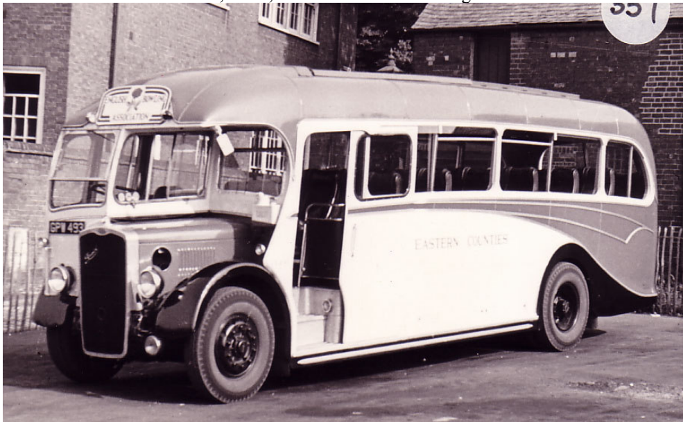
LS 493 (GPW 493) was the third vehicle to be classified as an LS by ECOC. LS 493 was a Bristol L6B with a Beadle 28 seat forward entrance coach body. Three such vehicles were delivered in 1949 and had a relatively short eleven year life with the company, all being withdrawn by 1960. The very attractive LS 493 is seen here on a private hire to the English Bowling Association in the early 1950s.
