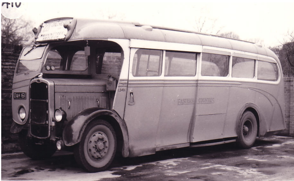
LS 1 (DAH 161) was the first vehicle to be classified as an LS by ECOC. LS1 (later LS 491) was a Bristol L5G with a 26 seat ECW coach body. She was the first of a batch of two such vehicles delivered in 1939. She saw 18 years passenger service with the company before withdrawal in 1957, 15 as a full coach. The LS class comprised an assortment of 93 Bristol L, LWL, LS & MW coaches dating from 1939 to 1964.
