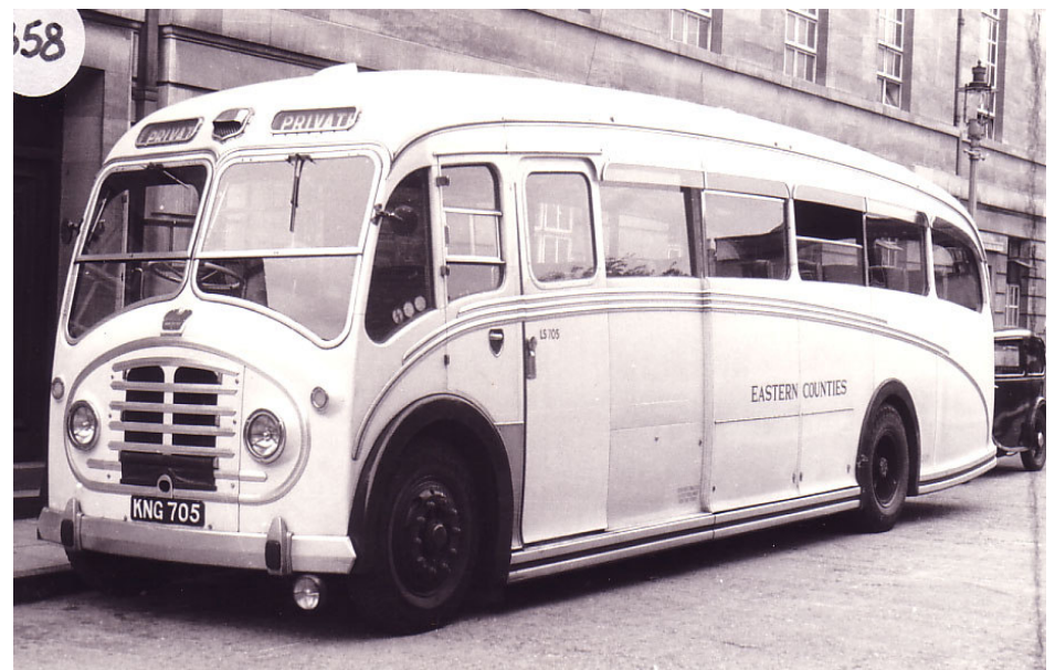
LS 705 (KNG 705) was a MkII ECW 'Queen Mary' bodied 35 seat Bristol LWL6B coach and was one of a batch of four such vehicles delivered to the company in 1951. She is seen here laying over on a private hire, possibly in London in the mid 1950s. She was withdrawn in 1966 after 15 years passenger service, 10 as a full coach.
