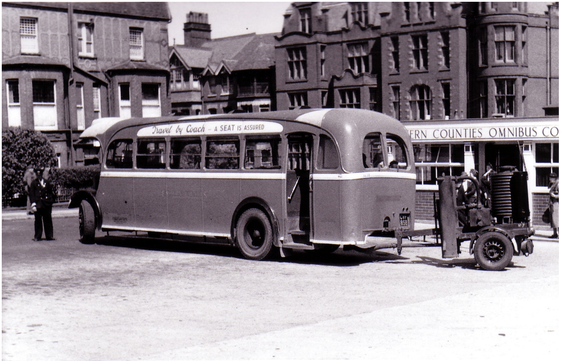
LL 58 (CVF 858) complete with 'producer gas' trailer, pictured here at Cromer's Cadogan Road bus station during the summer of 1942.
